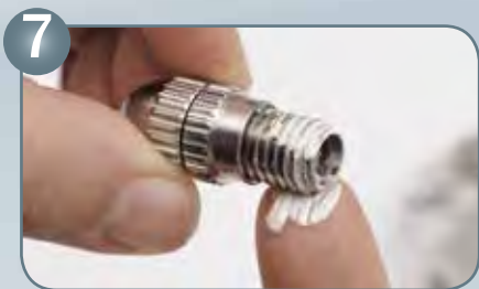
Grease thread of material flow control screw
