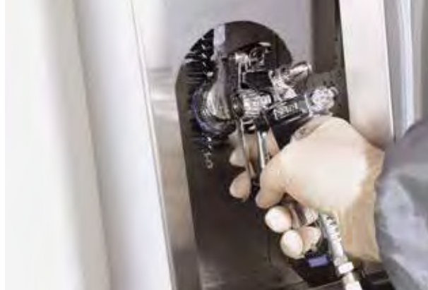
1. Cleaning of material passage and air cap
