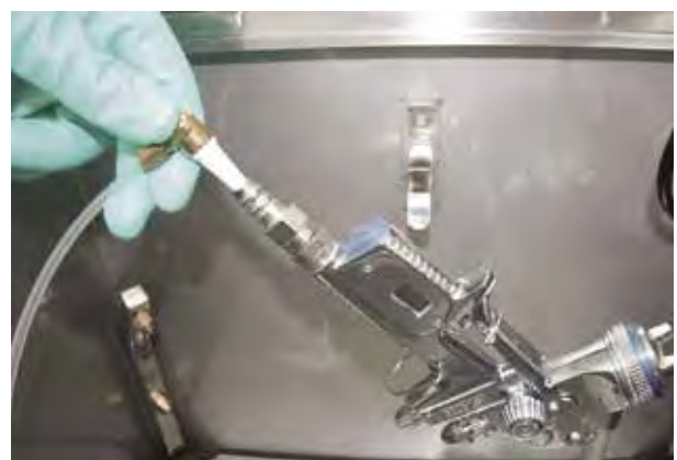
2. Connect air connection to air inlet
