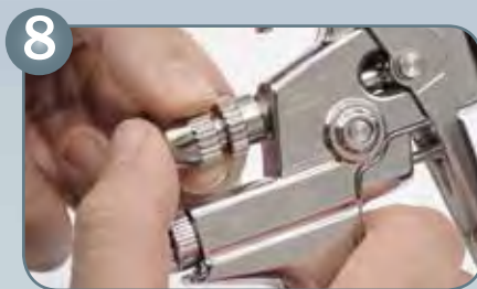
Install material flow control screw
