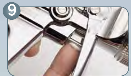
Grease visible part of air piston rod
