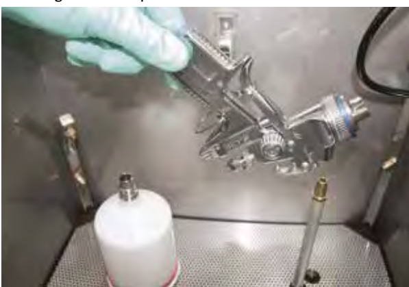
1. Insert gun in correct position
