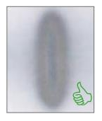
Clogged or damaged nozzle elements can cause faulty spray patterns. In most of the cases, these contaminations can be easily removed – the comprehensive SATA guide "Cleaning and Maintenance of Paint Spray Guns" demonstrates how: www.sata.com/firstaid.
